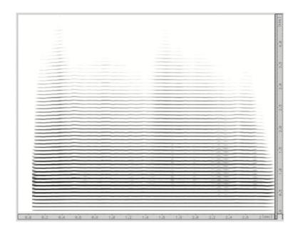
Figure 3: Trombone spectrograph
